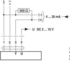
The 500  $\Omega$  resistor converts the 4 ... 20 mA current signal to a voltage signal DC 2 ... 10 V. Operating range set to DC 2 ... 10 V.
